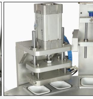
A Rotary Cup Filling Sealing Machine is a compact, automated system designed to fill efficiently and seal cups in a rotating table process, making it ideal for small to medium production runs in the food and beverage industry. It offers versatility in handling various cup sizes and materials with consistent sealing quality.
